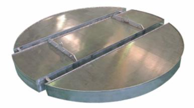
**Support Grids:** are typically made from wedge wire screens to retain media or catalyst allowing liquid or vapour to pass unhindered through the catalyst. This creates direct retention of media, removing the requirement for an intermediate layer of inert balls. Apollo Screens designs grids to handle the operating conditions of each application, taking the material requirements, load and temperature as well as the process licensor specifications into consideration.
