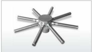
**Header Laterals:** are made from a series of screen laterals fitted to either a central header or hub, providing uniform flow through catalyst. Apollo Screens supply laterals and header laterals for Ion Exchange units, Sand Filters, Salt filters, PTA, jet fuel/kerosene sweetening units and many other processes requiring catalyst retention.
