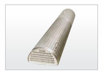
**Scallops:** Perforated scallops have been for over 30 years the standard method for catalyst retention in radial flow reactors. The main function of the perforated scallop is to protect the centre pipe from deformation during temperature spikes, sudden increases in pressure and coke build-up. The scallop has a twofold function:
